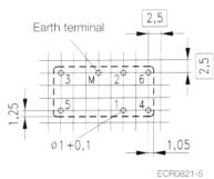
Pin arrangement suits 2,5 mm and 2,54 mm in acc. with DIN EN 60097 and DIN 40803
