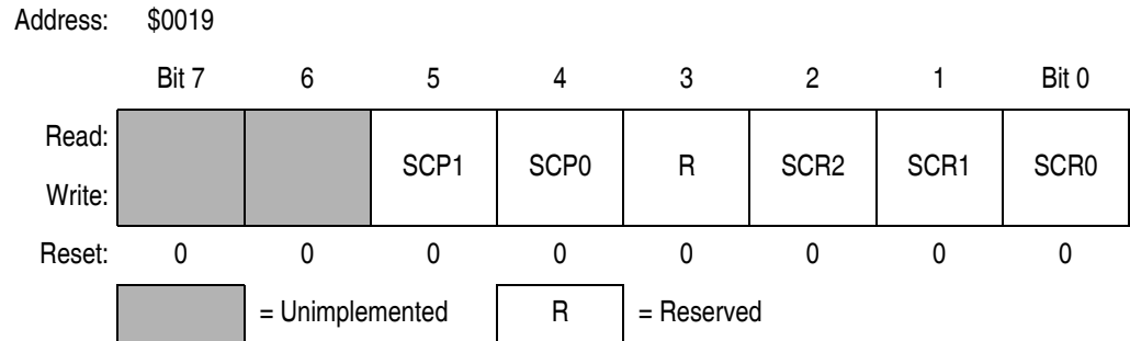
Figure 17-18. SCI Baud Rate Register (SCBR)
