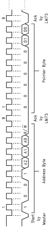
(b) Typical Pointer Set Followed by Immediate Read for 2-Byte Register such as Temp, T<sub>OS</sub>, T<sub>HYST</sub>
