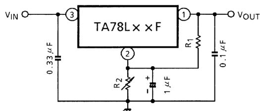
$$V_{OUT} = R_2 \left( I_B + \frac{V_{OUT}(\text{of IC})}{R_1} \right) + V_{OUT}(\text{of IC})$$
