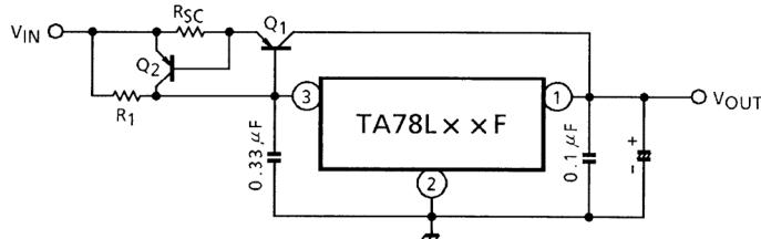
$$R_{SC} = \frac{V_{BE2}}{I_{SC}}$$
