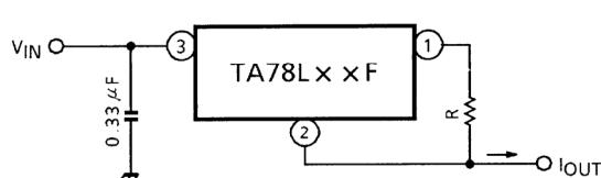
$$I_{OUT} = \frac{V_{OUT}}{R} + I_B$$
