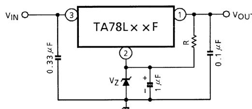
$$V_{OUT} = V_Z + V_{OUT}(\text{of IC})$$
