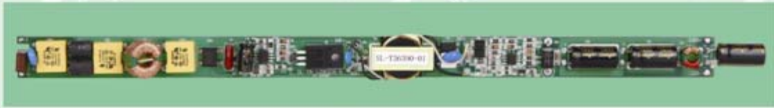
T5/T8/T10 Tube driver 18W
