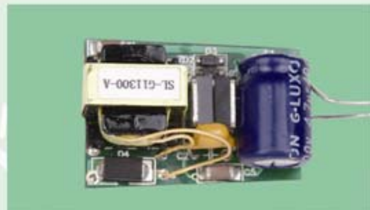
Isolated dimmable driver 3-6W
